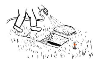
Now replace the soil, lay the turf on the soil and tread down. Everything will grow back faster if you water the soil and turf beforehand. After two to three weeks, you will not be able to see the system any more.
