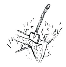
Use a spade to cut out a v-shaped pipe trench approx. 20-25 cm deep. When doing so, carefully remove the turf that you have dug out and dig out the trench. Remove any stones
