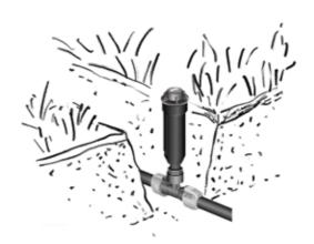
G Lay lines with sprinklers and components connected in the trench. All sprinklers, connecting points, and water connectors must be installed flush with the ground surface. The head including recessed grip should be above the ground for regular cleaning.
