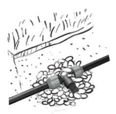
H The drain valves are installed at the lowest points of the system. On slopes, the height difference between the drain valves must not exceed 2 m. Install several drain valves on slopes if necessary. To improve drainage and to protect the drain valve underlay it with a seeping water drain packing (washed, coarse gravel, approx. 20 × 20 × 20 cm).
